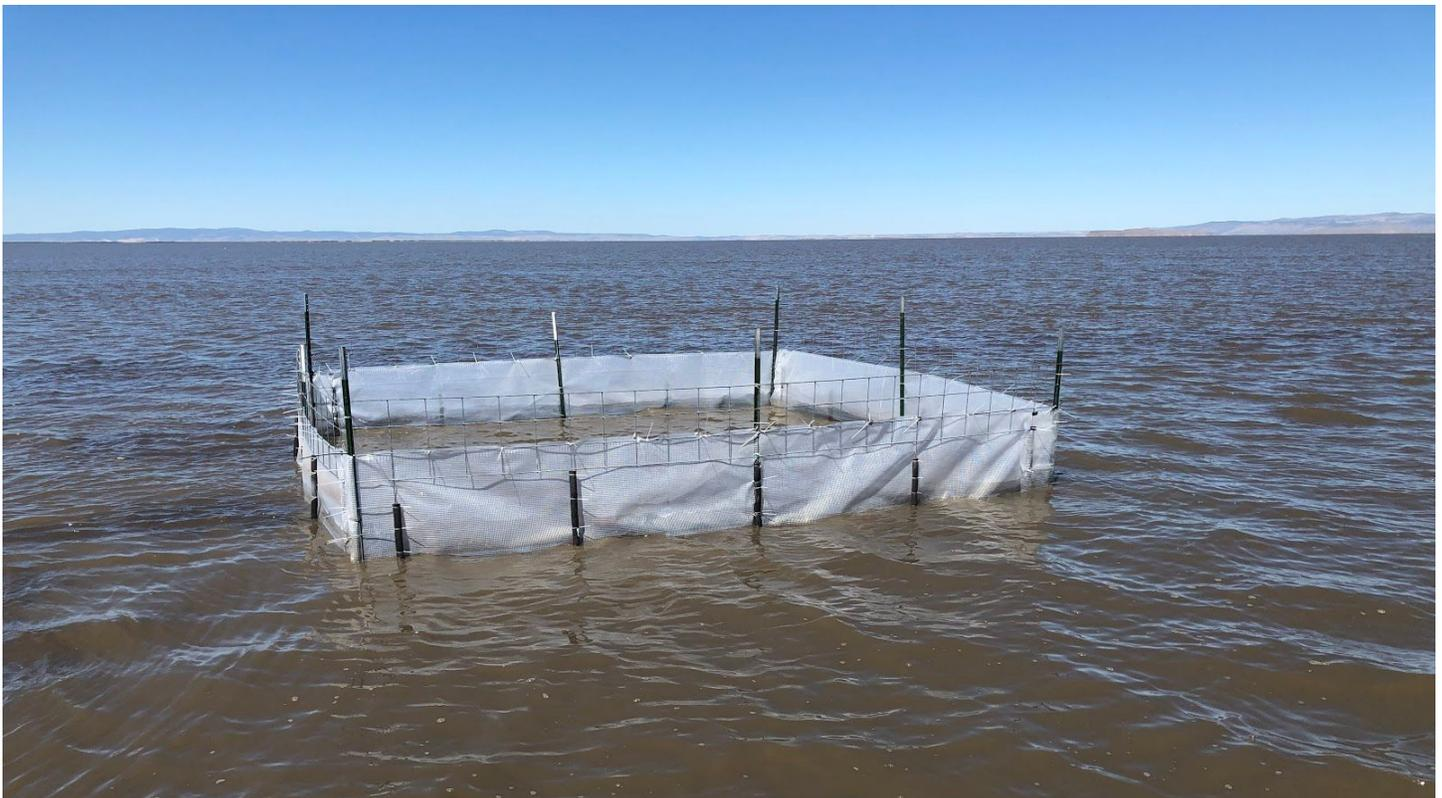
*Pictured: A mesocosm prototype structure in Malheur Lake made of PVC pipe and plastic sheeting.*
